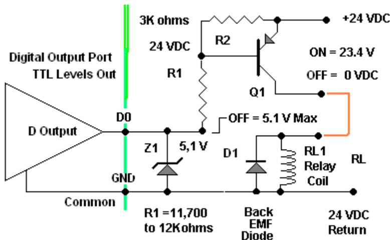
In either of the above cases, the relay and D1 diode could be replaced with a load resistor or active device. Then we would need to know how much current Q1 could source or sink. Typical coil resistance for "Ice Cube" type SPST 24VCD relay is 750 ohms.
