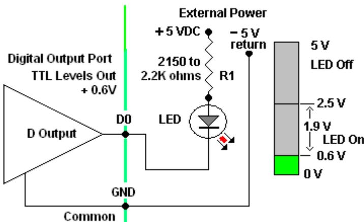
**Figure 2: Current Sinking**
